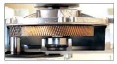
Oil-filled, totally sealed gearbox houses the brass helical gears delivering quiet positive power. The sealed gearbox eliminates contamination from dust and chemicals. Keeps going when belt and pulley systems have given up. More power. More reliability. Longer life.
